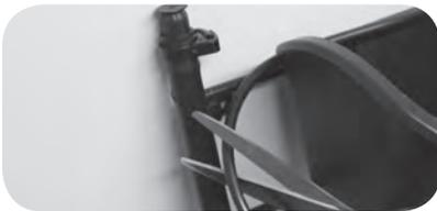
h) Cut the 4mm tube to the length to position the take off in the centre of the pot.
