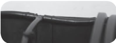
g) Use a 4mm tee piece to insert a take off for the first 2 pots and a 4mm elbow for the last pot. (Heating up the 4mm tube in the sun or hot water makes it easier)
