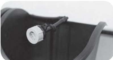
i) Cut a convenient length of 4mm tube to go from the 4mm tee or elbow and insert an adjustable dripper in the pipe and then push onto a tee or elbow.
