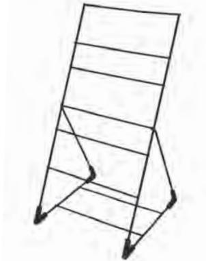
4) Secure the main panel by connecting the back stands with the plastic corners of the base. Clip the circlips on the main frame to secure the Free-Standing Planting Kit.
